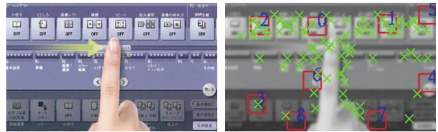
Fig. 7 Marker-less technology. An example of an image (left) used as a marker, and an image (right) with extracted characteristics (x marks).
